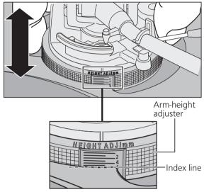
When checking the index line of the Armheight adjuster, check with your eyes on the same level.
